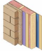
W05 Split Insulated Wood Frame with Mineral Wool and Stone Veneer Cladding
