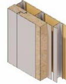
W15 Existing Masonry with Interior Spray Foam Insulation
