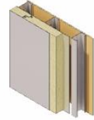
W16 Existing Masonry with Exterior EIFS Overcladding
