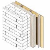
W15 Existing Masonry with Interior Spray Foam Insulation
