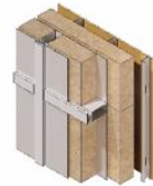
W08 Spandrel Panel with 3" Mineral Wool Backpan, Interior Insulated with Mineral Wool
