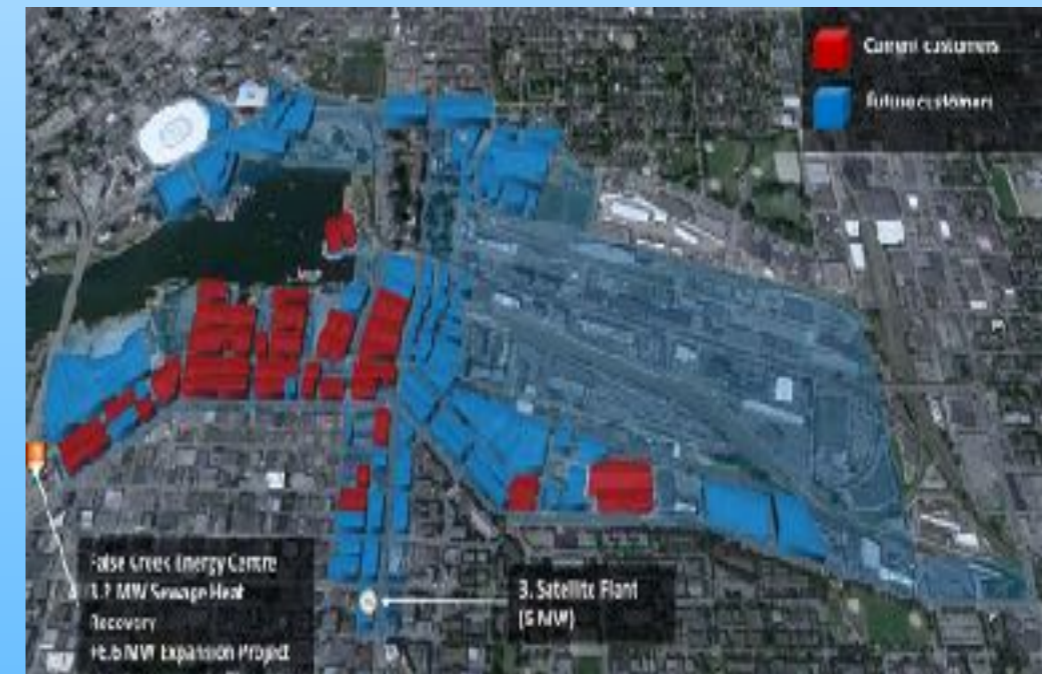
Wastewater energy reclaim for 37 buildings at False Creek in Vancouver, BC.
