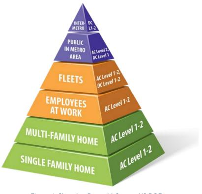
Figure 4: Charging Pyramid. Source: US DOE.
