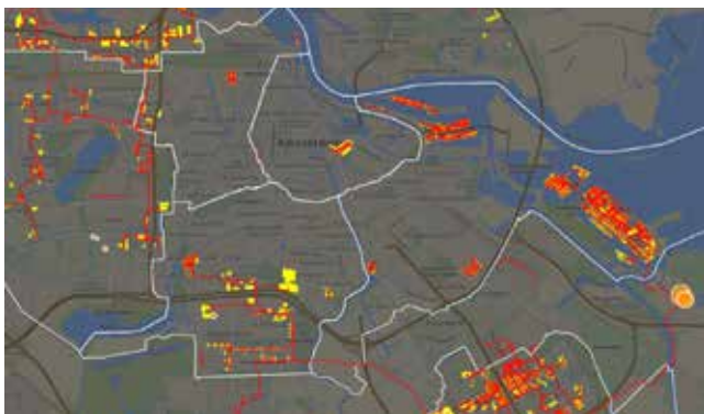
City of Amsterdam, Interactive Maps , 'Energy from waste incineration and waste heat'. Map showing the existing district heat network in Amsterdam (red) with connected load (yellow) and sources of waste heat (orange). Map data: © 2015 Google. www.amsterdamsmartcity.com
