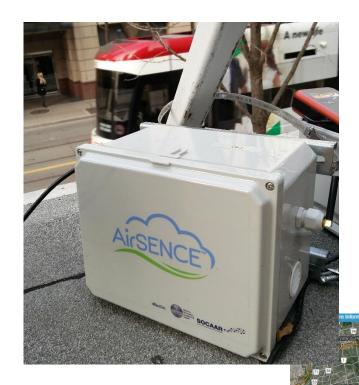
Array of sensors for: CO, NOx, O3 CO2 and PM
