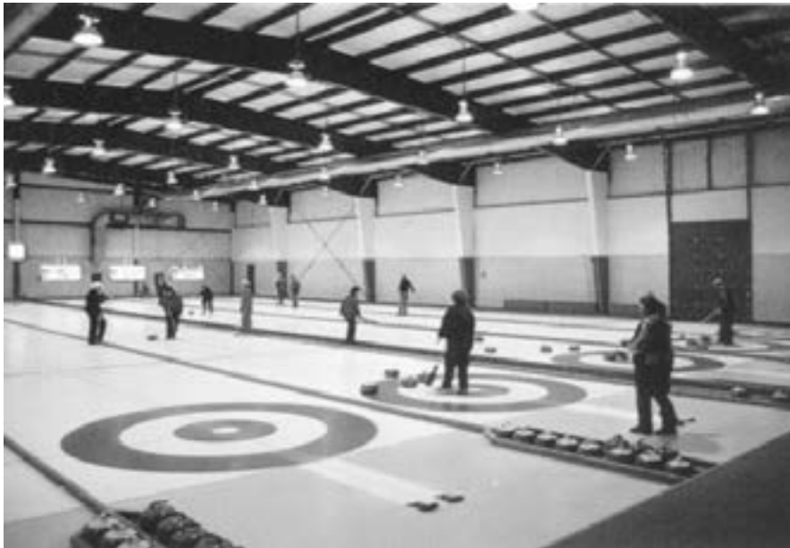
Changing to energy efficient metal halide lighting fixtures in this curling rink saved electricity to run the lights, reducing the amount of heat generated by the lighting. As a result, the savings gained from installing energy efficient lighting were offset by the additional heating required.
