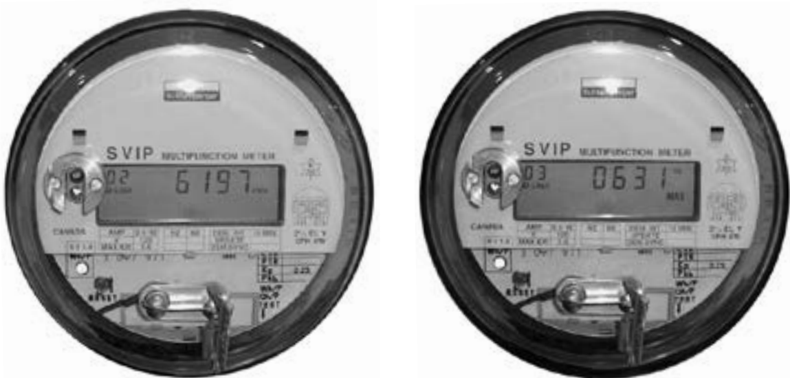
Front panel of an electronic meter for reading energy and demand. The meter is shown in energy consumed mode (left) and in demand mode (right). The tag below gives the multipliers for this meter.
