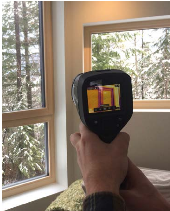
Photos: Left: Thermal image being taken during a builders' workshop in Fernie; the home is designed to achieve at least Part 9, Step 3.
