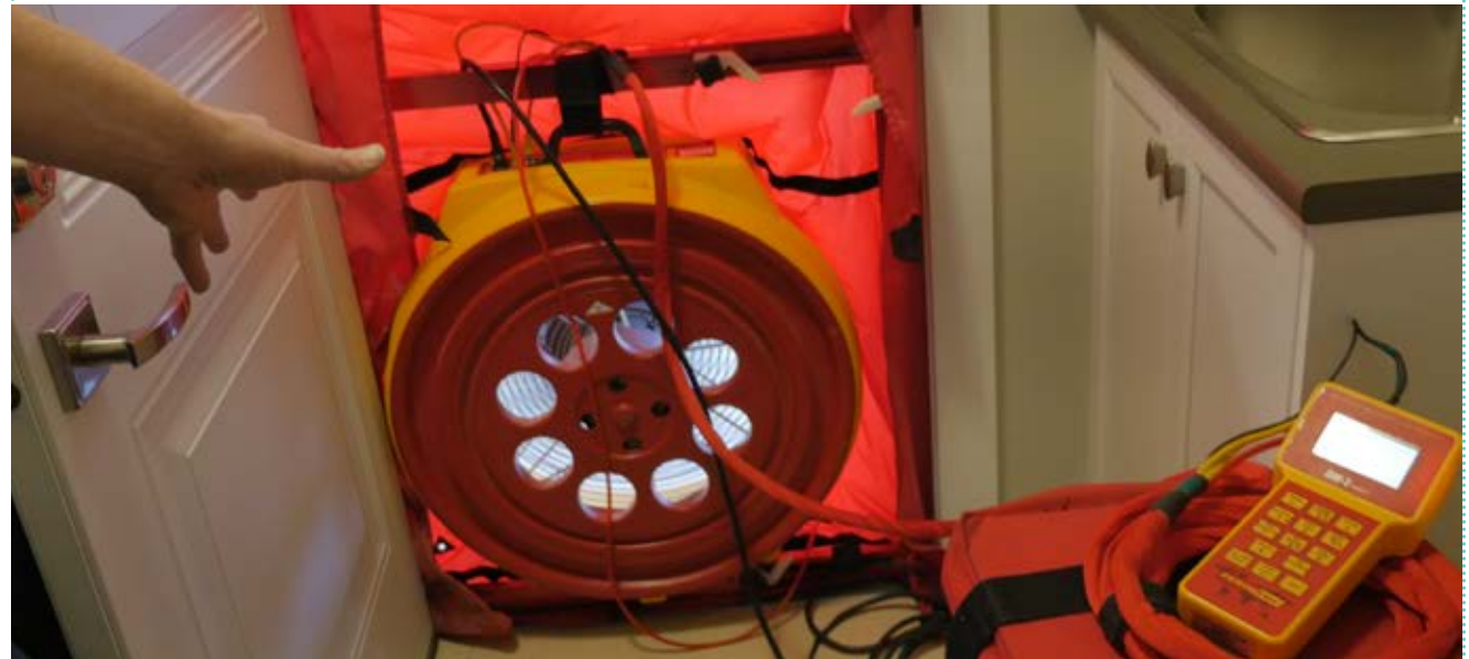
Figure 8: Blower door test in action
