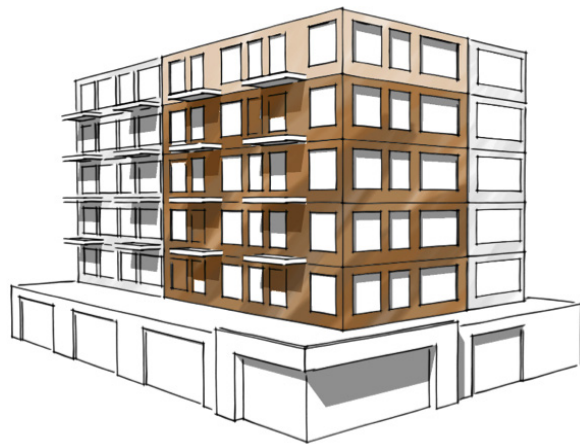
Figure 20: Compact form helps to minimize thermal bridging through the building envelope
